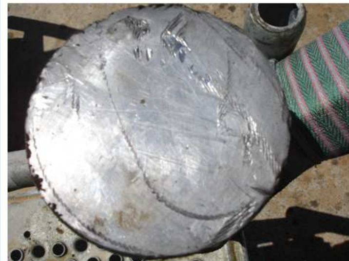
12-Mar-2011: 3.8" LIB after driving fish 6m down from 3397mtbf
