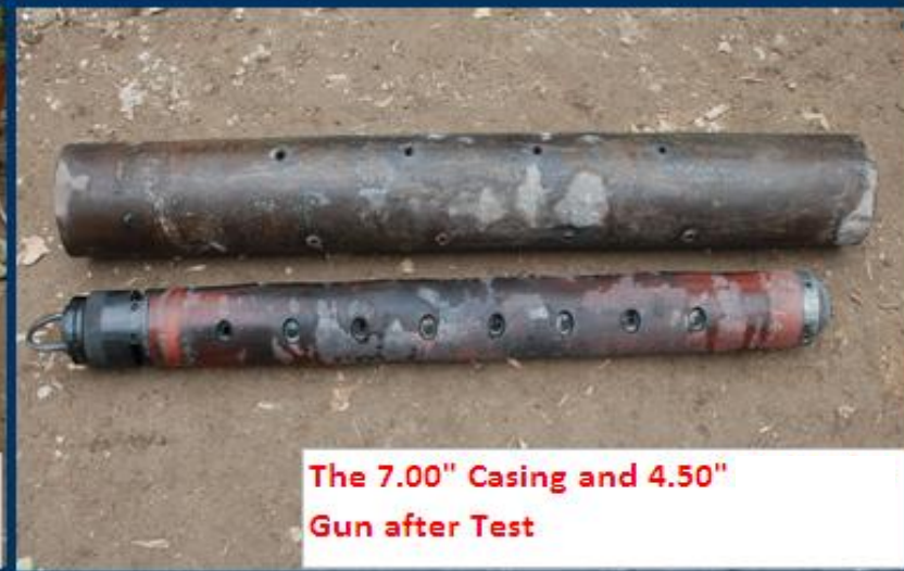
Debris of the Gun, the Casing and the Concrete after perforating
