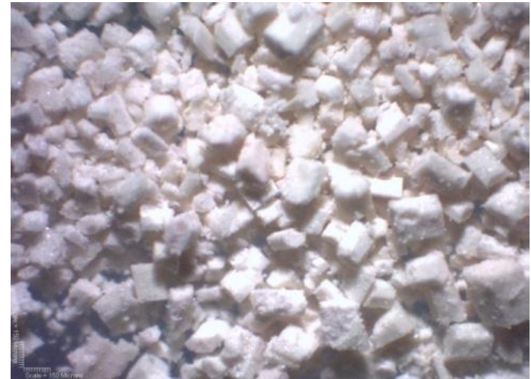
PYX crystalline structure (tailored for oilfield products)
