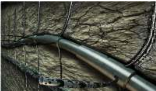
Fishbones Sub with Production Valve and Needles
